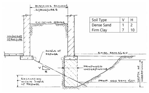
Angle of Repose Illustration Illustration of underpinning proposed to be constructed within the angle of repose of an adjacent footing.
